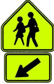
The School Crosswalk Warning assembly shall be installed at the marked crosswalk, or as close to it as possible, and shall consist of a School Advance Warning sign supplemented with a diagonal downward pointing arrow plaque to show the location of the crossing. These signs are not to be used at marked crosswalks other than those adjacent to schools and those on established school routes. The School Crosswalk Assembly signs also shall not be installed on approaches controlled by stop signs.
